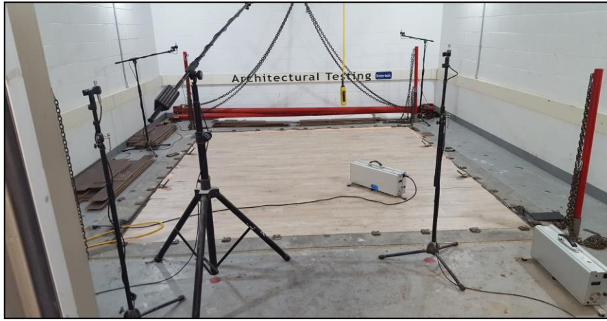
Source Room View of Test Specimen Installation
